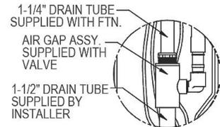
**SANITARY FREEZE-RESISTANT VALVE GROUND INSTALL DETAIL**
